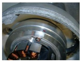
Should you once disassemble the stator unit, make sure during re-assembly to bring the coil holder plate into the same position. Otherwise the ignition marking will not be valid any more.
