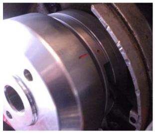
Take the rotor carefully off again without changing the crank's position.
