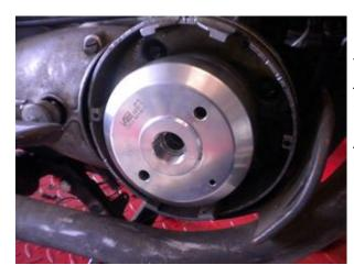
Place the rotor loosely onto the crank and check that it may move freely above the statorbase.
