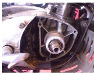
Further work is not at the engine block itself, but at the plate serving as a carrier of the alternator.
